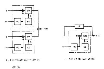
Fig. I-1 FM sound generation expressed by unit cell design
